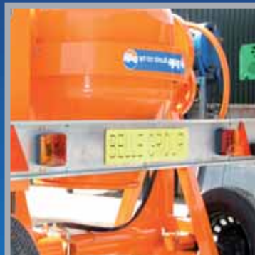
Integrated Lighting Board
